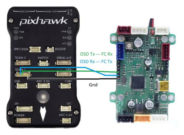
OSD works with fixed transmission parameters: 8 bit data, 1 bit stop, no parity, and default 57600 bps. Transmission speed can be set to 19200, 38400 or 57600 bps using FPV\_manager application (page OSD->settings, in **MavLink USART** box).
