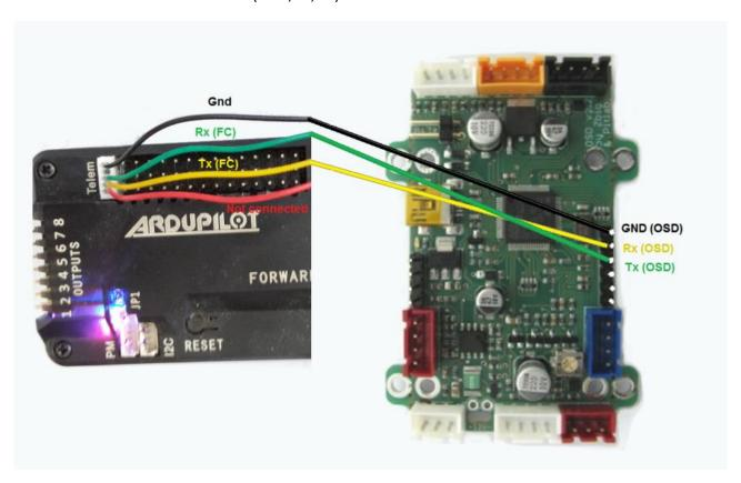
To connect Pixhawk use its spare telemetry port, and connect OSD as follows:
